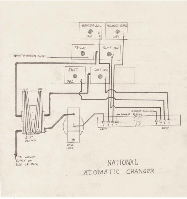
Please note: The tracker bar connections shown in the above diagram do not coincide with the tracker bar scale published by Art Reblitz and that is generally recognized to be accurate.
